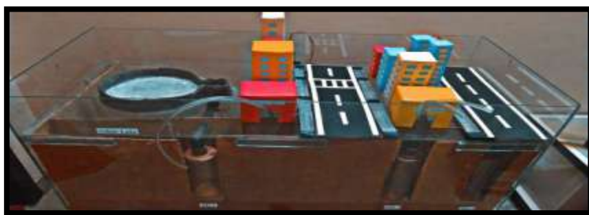
Fig. 4. Physical working model demonstrating floodwater diversion.
